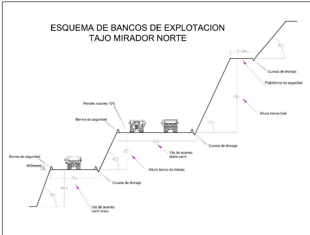
Figure 5-8 Schematic of operating banks of the Mirador Norte Pit
